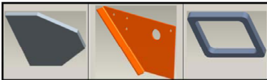
These were the gussets and brackets that were applied to the rear lift gear to support the high areas of stress.
